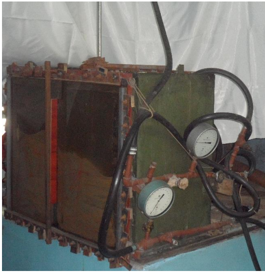
Figure 2: General view of the laboratory facility to study soil underwater washing processes by a water jet.
